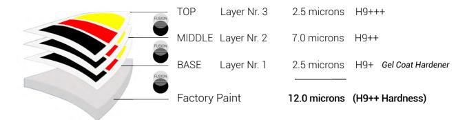
Trinity Fusion Ceramic Coating is based on silicon-nitrogen polymers and ceramics derived from reactions of dichlorosilane with ammonia. This chemical platform is more expensive but gives far much more durability and is a must to meet customer expectations / or to avoid customer complaints.
