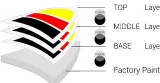
Trinity Fusion Ceramic Coating is based on silicon-nitrogen polymers and ceramics derived from reactions of dichlorosilane with ammonia. This chemical platform is more expensive but gives far much more durability and is a must to meet customer expectations / or to avoid customer complaints.
