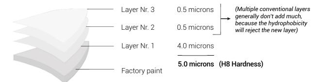
New cars are delivered with a standard factory soft or hard paint. (most glossy cars have soft factory paint). Keep in mind that soft paint is not a good base, this will result in a less hardness of the first layer.
