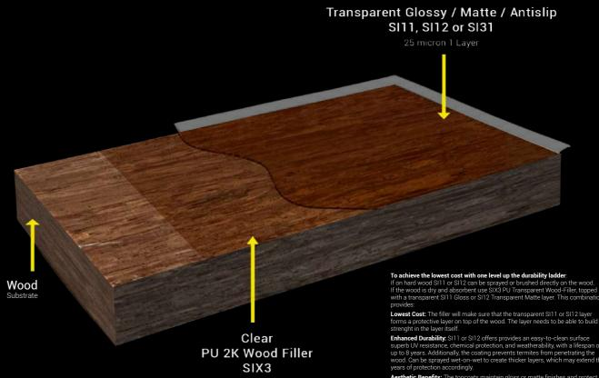
For areas where slip resistance is needed, apply SI31 AntiSlip without compr mising protection or appearance.
